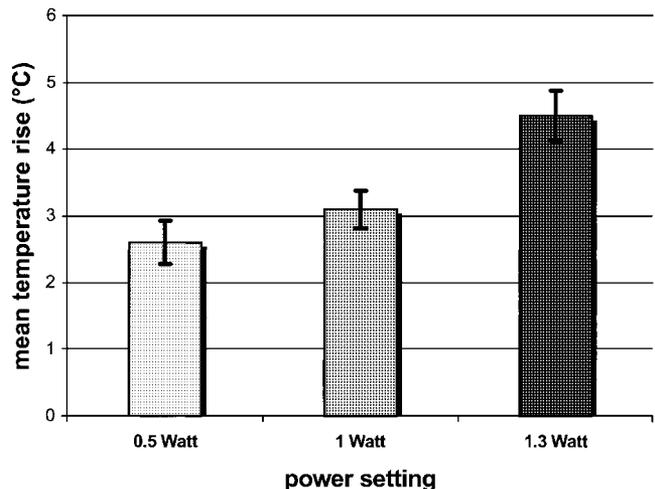
Fig. 4. Mean temperature rise during irradiation at power settings of 0.5, 1, and 1.3 W.
