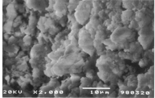
Fig. 3. SEM image of the root canal wall after irradiation at 1.3 W, 5 × 5 seconds. Longitudinal cut through the root, magnification × 2000, 20 kV.
