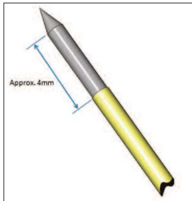
Figure 6: Diagrammatic representation of the 400-micron tapered and stripped tip used for this laser study
